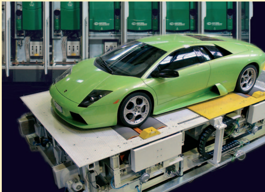
Unidrive's integration flexibility is making it the "standard" drive in automobile plants around the world. The rolling test rig performs simulated road testing of front-wheel, rear-wheel and four-wheel drive vehicles, checking motor, brake, and gearbox performance and road-noise decibel levels.
