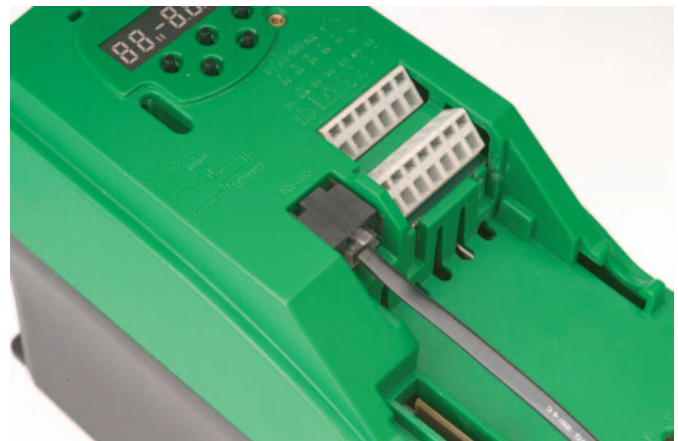
Commander SK showing connection to the serial port
